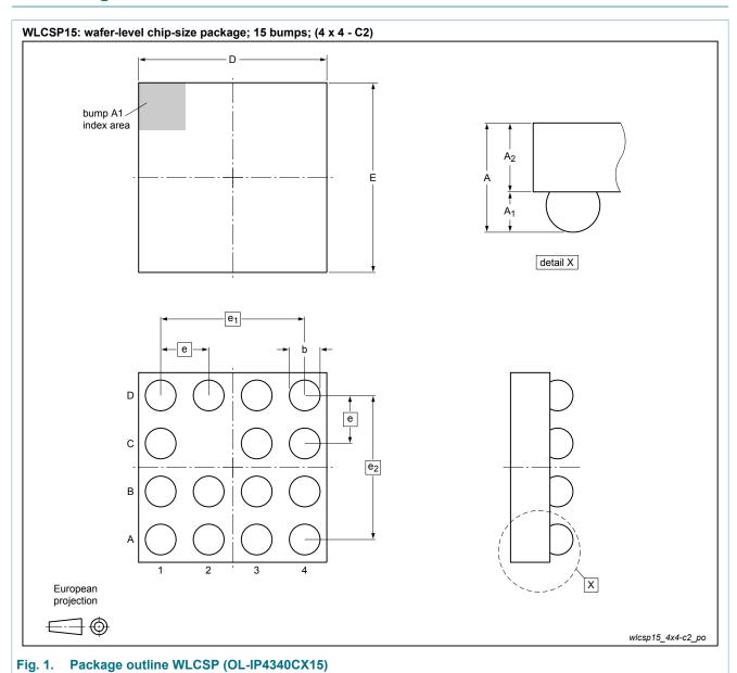
wafer-level chip-size package; 15 bumps; (4 x 4 -C2); 0.4 mm pitch; 1.56 mm x 1.56 mm x 0.47 mm body
